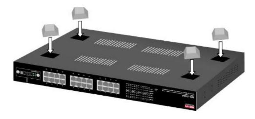
Figure 2-4. Attach rubber feet to each corner on the bottom of the Switch
